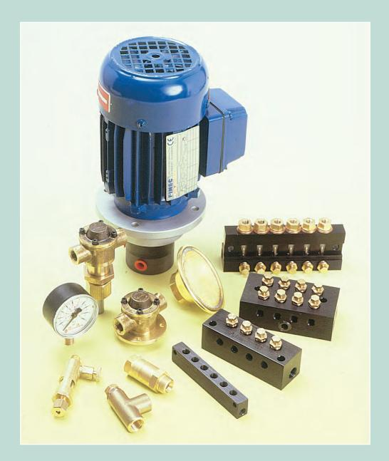
Ontinuous oil lubrication systems can employ various mechanical or electrically operated pumps to give a relatively low pressure but constant flow of lubricant to bearing journals, slideways or gears in any self-contained piece of machinery.
